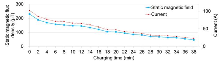
Fig. 1. Time variation of magnetic field during quick charging (ex. Type A, SOC 20%, in contact with charging cable)
